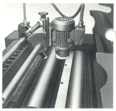
\*Built-in Grinder and Jointer A further aid to productivity. Feed speed is increased to 30.5 m/min (100ft/min) and cutters can be jointed and ground without removing them from the machine, a saving in 'down-time'. Produces a better finish i.e. 12 cutter marks per inch can be obtained at a feed speed of 26m/min (85ft/min).
