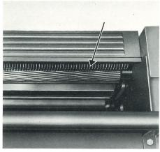
Anti-kickback Fingers Fitted as standard for increased safety. Prevents timber "kicking" back and possible injury.
