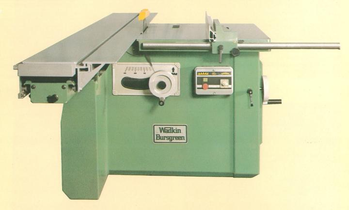
This superbly designed variant of the CP12 is a powerful, robust sliding table dimensioning machine for high accuracy work on solid timber, with a capacity up to 135mm depth of cut. The 400 x 1300mm free running sliding table provides the ability to undertake accurate crosscutting and mitring work using an adjustable mitre fence.
