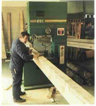
The EEC – is designed primarily for sawmilling but in view of its versatility will suit a wide range of uses. Examples of typical feed speeds for softwood ranges from 12" deep at 20 ft/m to 2" deep and below at 100 ft/m.
