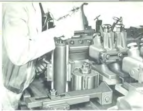
Straight jointing on side head.
