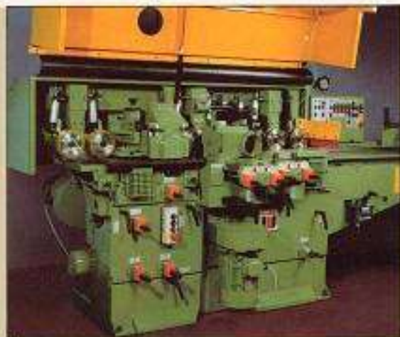
△ GD5 from outfeed end with cover open showing mechanical digital readouts to all main positions.
