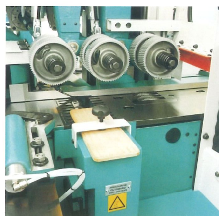
Short infeed table with the unique Wadkin PHT nip roller system giving excellent feed characteristics
