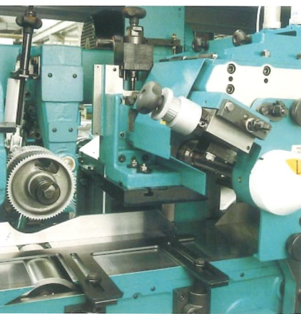
Top head manual jointer - combination straight and profile jointer
