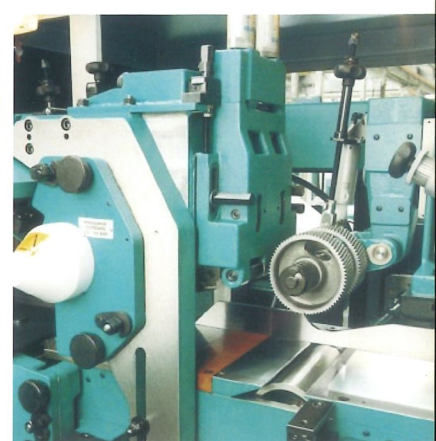
Top head chipbreaker unit is pneumatically controlled. Also highlighted is driven bed roller between top heads
