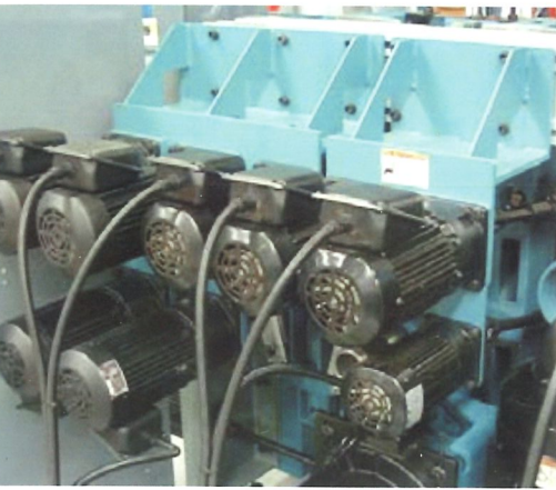
Individual motors and gearboxes provide drive for each feed roller
