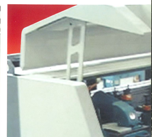
An integrated close fitting safety cover ensures full CE capability with exceptional sound absorption
