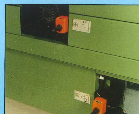
Dial-a-size setting for tenon thickness, bottom shoulder height and shoulder stagger.
