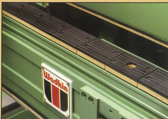
△ Rubber top track pads for panel and furniture components.
