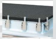
■ 4 pneumatically lowerable Aluminium stop cylinders (in front right)
