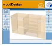
Simple 3D construction of furniture including a parts list output and export of cut plans
