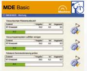
■ Machine Data Recording collecting and evaluating machine states via time meter and event meter
