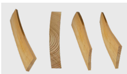
Blocks with longitudinal/latitudinal deformation, cupped or warped
