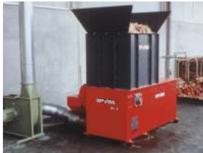
WL 6 series shredder with a connected extraction system
