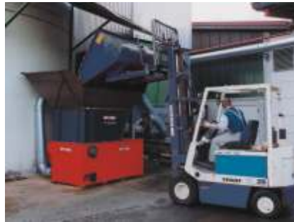
WL 6 S series shredder, material loading by fork-lift truck with tripper
