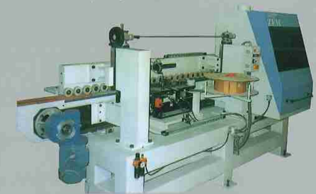
Insertadora de Burlete Machine for cutting kerf pocket and inserting weather strip
