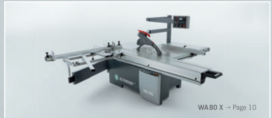
Altendorf WA 80 X with motorised rise/fall and tilt adjustment of the main saw blade and motorised adjustment of the rip fence.
