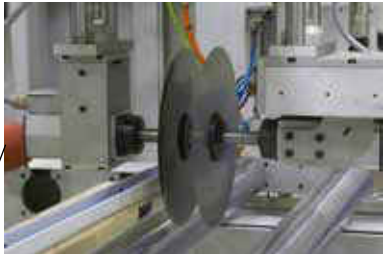
Separation cut with double saw
