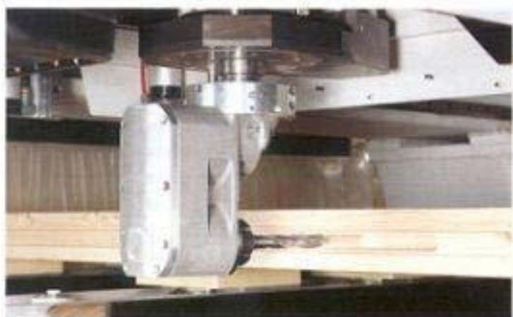
■ Mortising for key-lock.
