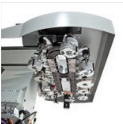
Chain-type tool magazine 22 positions and 44 positions (opt) with 180 mm between centres.
