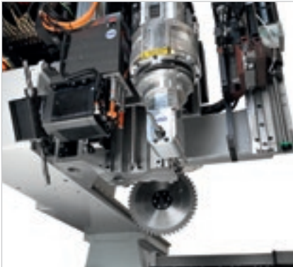
Electrospindle, 19.2 kW. FlexyWood PLUS. Unit 3+1.
