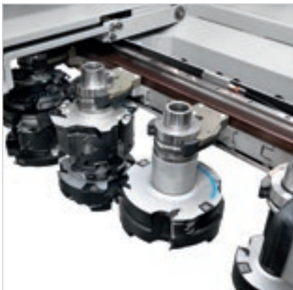
New metal-reinforced collet for loading tools up to 10 kg.
