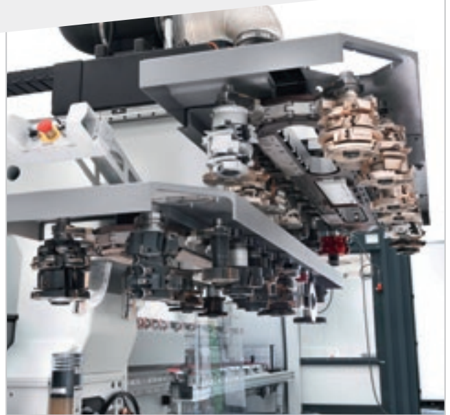
Dual-level chain magazine with a total of 44 places.
