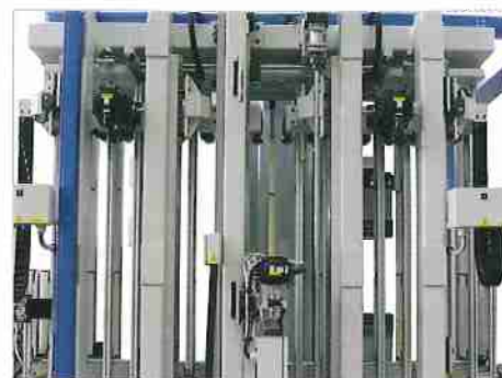
Opposite side of the machine equipped with sawing unit and self-selecting drilling unit.
