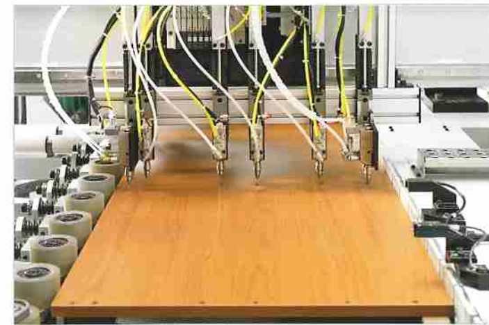
Detail - machine Mod. GDM for glue insertion in holes and along the milling for the back.
