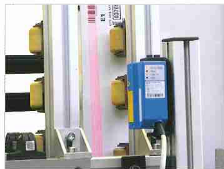
Detail of barcode reading on the panel during machine entry.
