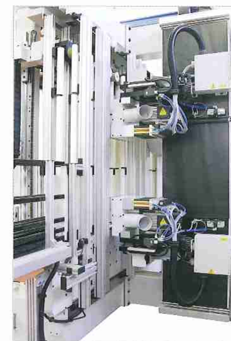
Column equipped with two self-selecting drilling units.
