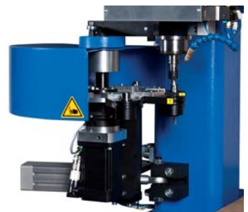
Tellerwechsler 8-fach, optional 8-time Disk type tool changer, optionally
