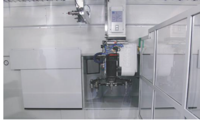
Tool changer magazine; 16 stations
