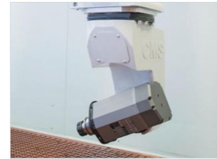
CX5 operating unit for continuous 5-axis interpolated machining
