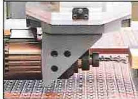
CNC-controlled horizontal electrospindle.
