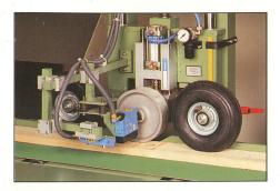
Even if there is slip between timber and infeed, no length inaccuracy will occur as the length measurement is done by an independant measuring wheel free of slips. Precision under all circumstances!
