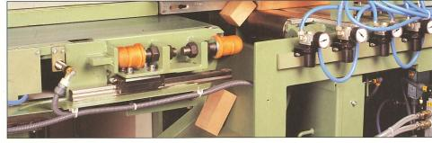
In the OptiCut an automatic separating shaft is integrated in close distance to the saw. Waste and good pieces are separated with 100% security. No piece of waste can find its way into the assorted good pieces. Dimter patent!
