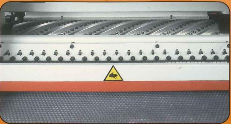
A simple system to moves infeed support rollers sideways provides access to the front of the planer and facilitates maintenance operations, knives rotation and changeover.
