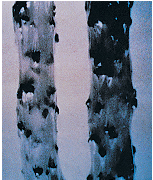
Figure 1. Magnified Picture of Grit Containing Tynex® A
