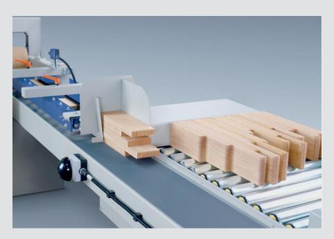
By the modular design of a finger jointing line you can determine the degree of automation yourself. No matter whether you wish to operate a manual, semi-automatic or full-automatic line: Depending on the requirements GRECON recommends the right degree of automation.
