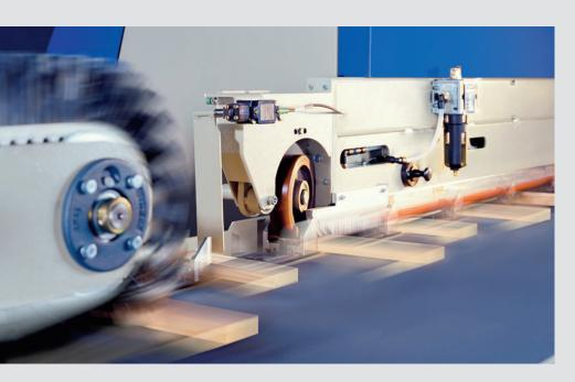
The horizontal single timber shapers from GRECON are the quickest equipment available on the world market. Up to 180 parts per minute in continuous operation and 12 pressing cycles per minute turn this line to a production giant. High-performance components, as the automatic feeding system, can be integrated in addition. Also cutting tool systems with a diameter between 228.6 mm and 266.7 mm (9 to 10.5") may be operated.
