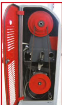
stabiler Riemenantrieb solid and smooth belt run
