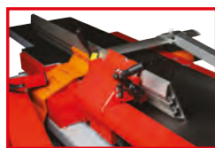
stabiler, schwenkbarer Abriechtanschlag accurate, tilting planer fence
