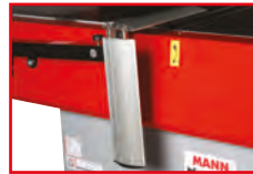
klappbare CPS Hobelwellenabdeckung CPS cutter block protection
