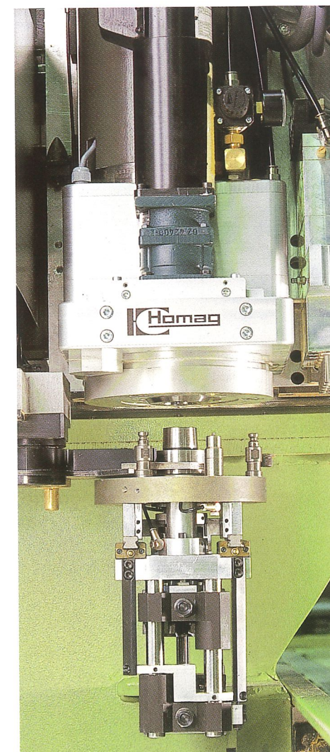
Main spindle with universal interface.
