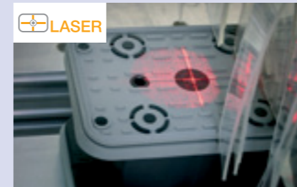
Suction cups are displayed using a laser beam (cross hairs). The workpiece contour can be "travelled" as a positioning aid for freeform parts.
