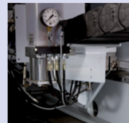
Covered linear guides with closed guide carriage and integrated central lubrication of all axes. Closed energy chains to protect against damage to cables and hoses.
