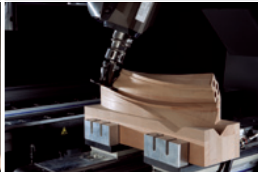
Routing of a stair hand rail
