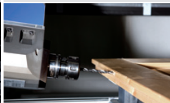
Step drilling for drill-in hinges
