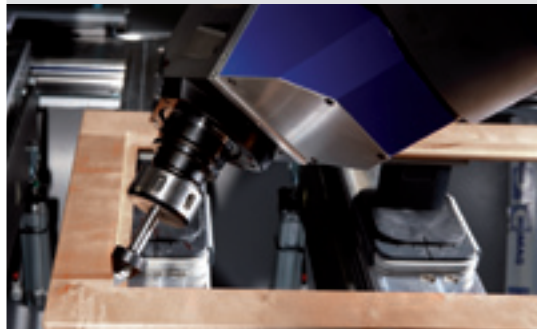
Square corner routing for a glass rebate
