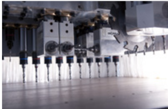
High-speed drilling technology with grooving saw
