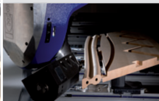
Holes for paling at narrow angles
