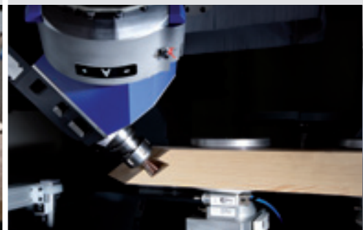
Routing of a dovetail joint for upright / transom constructions
