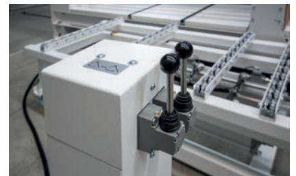
Operating the cabinet uprighter: By simply pulling on the lever, the cabinet uprighter aligns the pressed cabinet.
