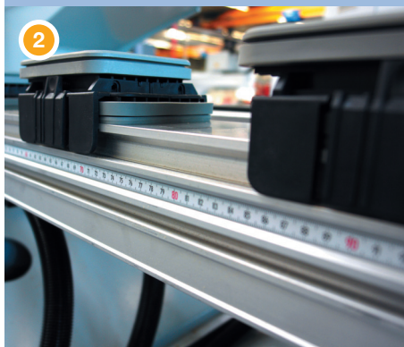
Tubeless vacuum clamping system
