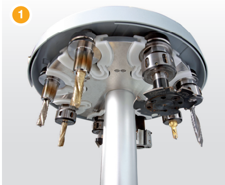
■ 8-fold tool changer moving in X-direction
