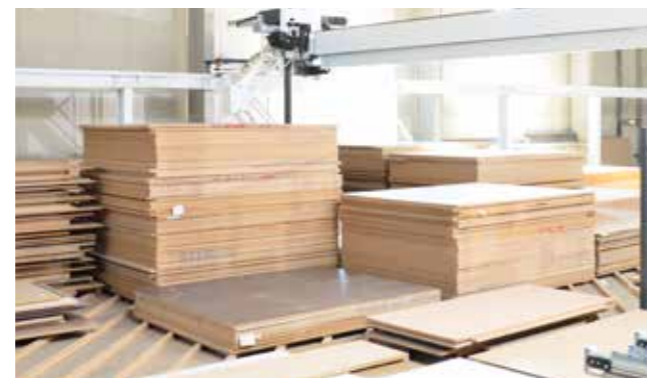
A lot of space for different kinds of material The STORETEQ S-700 offers the largest extent among the HOMAG storage systems with span width beyond 16 meters.
