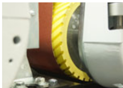
Optional Profiled contact rollers made of: ▪ Steel ▪ Rubberized in different Shore hardnesses
