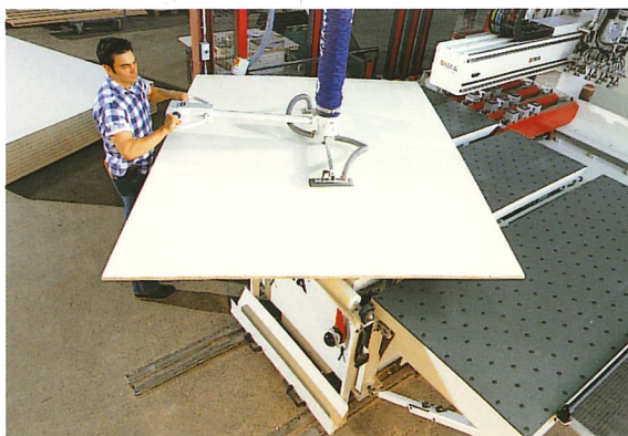
Feeding with vacuum lifting unit
