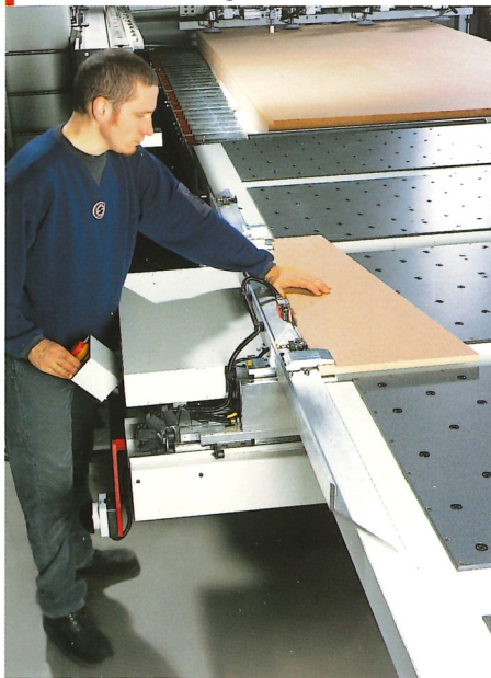
Positioning stop system for individual cutting to size and machining
