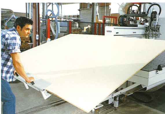
Feeding with a tilting device
