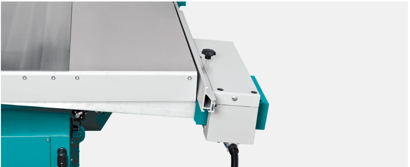
T7x stop with 1,350 mm cutting width
