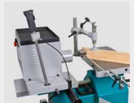
Standard feature: One-hand operation and excenter clamping
