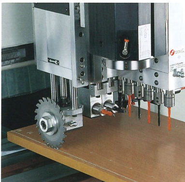
Sawing unit for grooving and cutting operations. Grupo sierra para ranuras y cortes. Zaagunits in diverse uitvoeringen.
