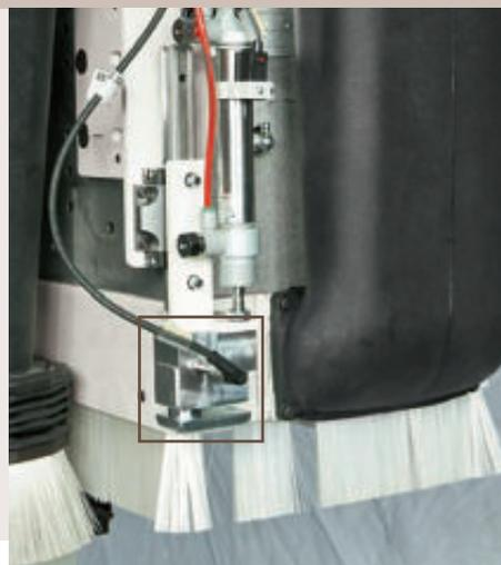
◉ Absolute precision in routing with the automatic measuring of the effective thickness of the panel in process and the length of the tools.
