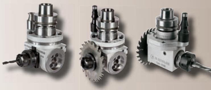
**VECTOR, 0/360° numerically controlled rotating continuous axis**, to execute, transversal and inclined borings and in respect of the panel's surface, utilising angular head. It can make without any problem also **interpolating routing operations** thanks to its body with **mechanical displacement extremely rigid and exact**.
