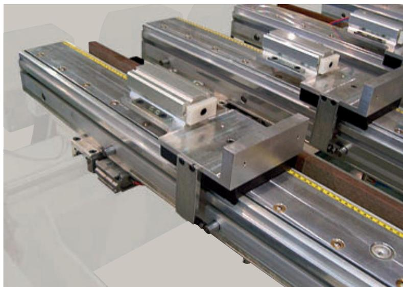
Studied with different dimensions, geometries and heights, the vacuum cups, are able to follow the shapes of the pieces to work in a such way to concentrate the vacuum only where it is necessary, increasing the locking efficiency of the pieces.
