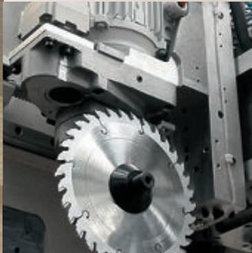
Boring unit group to work any type panel, with automatic rotation of the blade 0 to 90 ° operated from the CNC numerical control.
