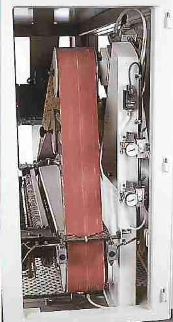
*Vista lateral grupo patín transversal. *Lateral view of the transversal pad group
