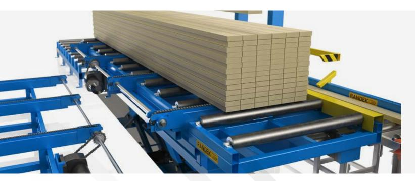
• For handling and feeding of entire piles of timber the saw and timber picker can be equipped with a modular handling system. The system can be configured according to customer requirements
