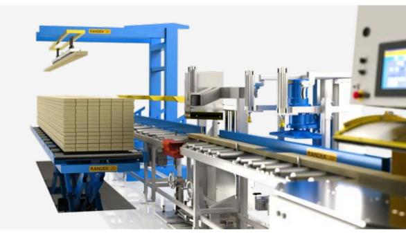
The timber picker picks timber with two vacuum pads from the timberpile and places them onto the infeed bench. Positioning of the pads is made with sensors placed on the picker. The timber is placed on a elevator and lowered to the infeed bench. The operator is given the possibility to flip or slide the timber down on the rollers. This option is available for roof truss producers who want to align their timber with the timber's natural curve to the roof truss.
