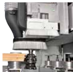
The rear routing unit with independent Y-axis is equipped with double Z-axis for 3 / 4-axis electrospindles + drilling unit.
