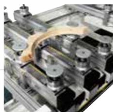
MATIC worktable: The bars and bases are moved using a rack and pinion direct transmission system and have independent motors for fast and precise positioning of vacuum cups and pneumatic clamps.
