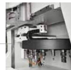
The 16 positions front circular store is ergonomic and compact. It is accessible from the machine front and prevents the machine footprint increase.
