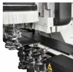
The rear chain store characterized by high capability and reduced dimensions allows to manage up to 48 heavy and large tools.
