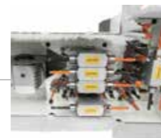
Drilling unit with independent spindles as well vertical as horizontal, and rotation speed up to 8000 rpm.
