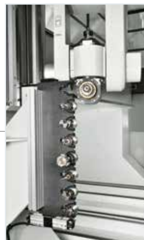
Linear tool store anchored to the upright of the gantry.
