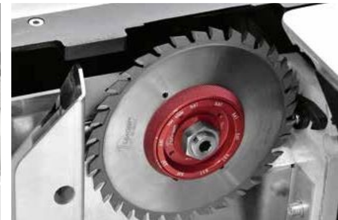
Expandable scoring blade Manually expandable with variable thickness from 2,8 to 3,6 mm. 120 mm blade diameter.
