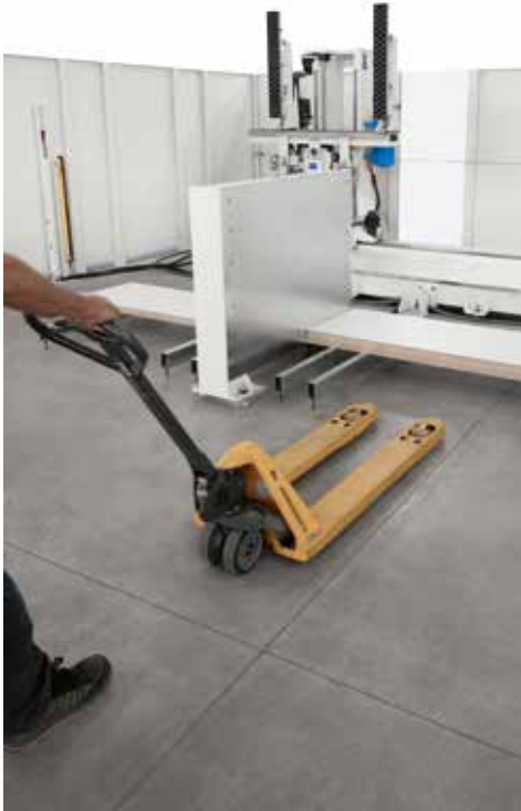
Two stations; one for loading and one for unloading, easily accessible even with a forklift truck.
