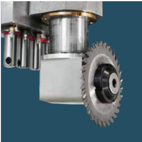
Easy grooves machining on the sides of the furniture thanks to the integrated blade unit.
