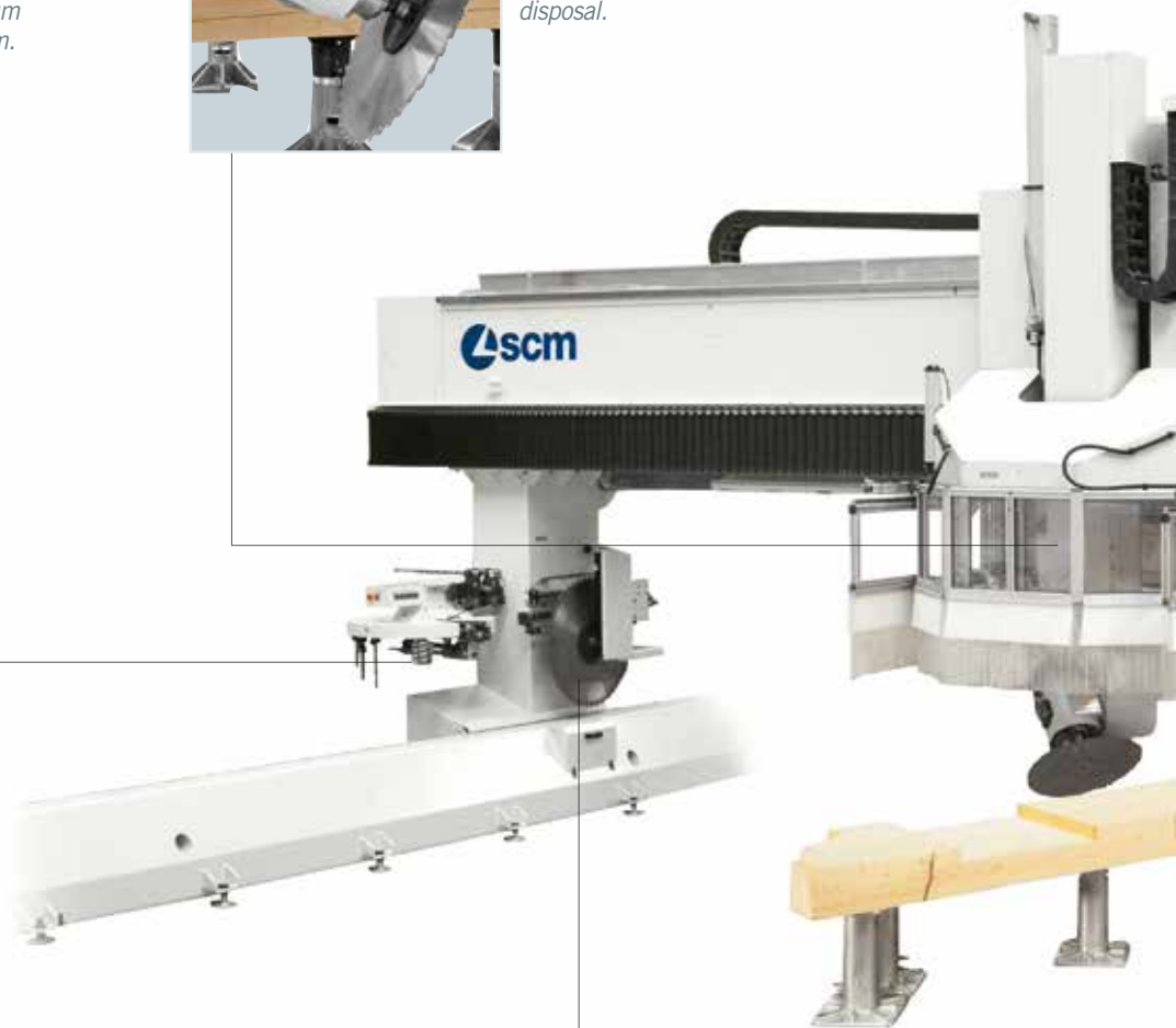
Main 5-axis machining head unit with dedicated extraction system for a complete dust disposal.
