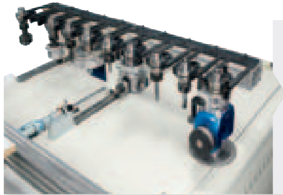
TR8, TR10, TR12, TR13 tool changer Positioned on the machine base. No problems even with large dimensioned tools.
