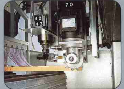
Fixed disc cutter along "X" direction (160 mm max. diameter).
