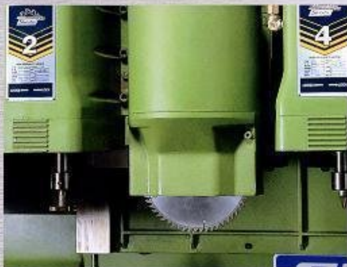
Center Saw (0, 90, 180, 270deg. Rotation)
