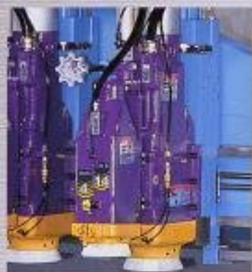
Piggyback Router 30,000rpm
