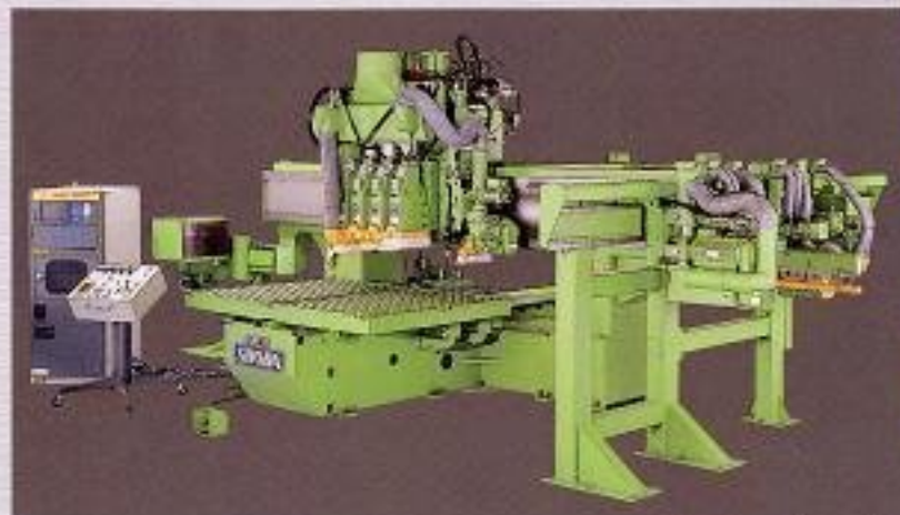
NC Router with A.H.C.(Auto Head Changer)
