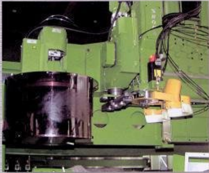
NC 360 deg. Rotation ATC (8/16 tools)
