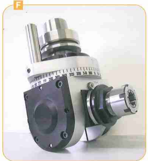
ISO30 Pinza ER25/32 HSK 63F Pinza ER25/32 6000/12000 rpm
